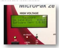
Under normal circumstances, the other boards will match the Display and Communications Processor Board and there will be no fault reported. If the version of software on one of the other boards does not match the display board, a fault will be displayed. This indicates that software needs to be updated on one or more of the other boards. The following picture is an example showing the fault message.
