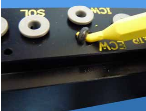
Remove the o-ring by using a non-metallic pick.
