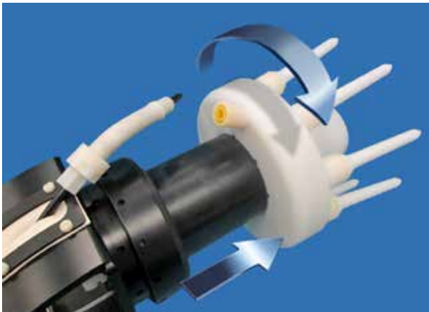
Grasp high voltage ring from the front and twist counter clockwise 10-15°. Slide the ring and probe forward off the applicator.
