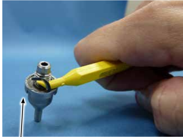
Orifice size engraved on this surface
