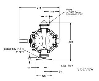
BOTH SUCTION AND DISCHARGE PORTS ARE AVAILABLE WITH 1" BSPT TAPERED THREADS (41-818823 STAINLESS STEEL ONLY)
