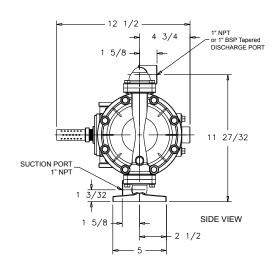
BOTH SUCTION AND DISCHARGE PORTS ARE AVAILABLE WITH 1" BSPT TAPERED THREADS (41-818823 STAINLESS STEEL ONLY)
