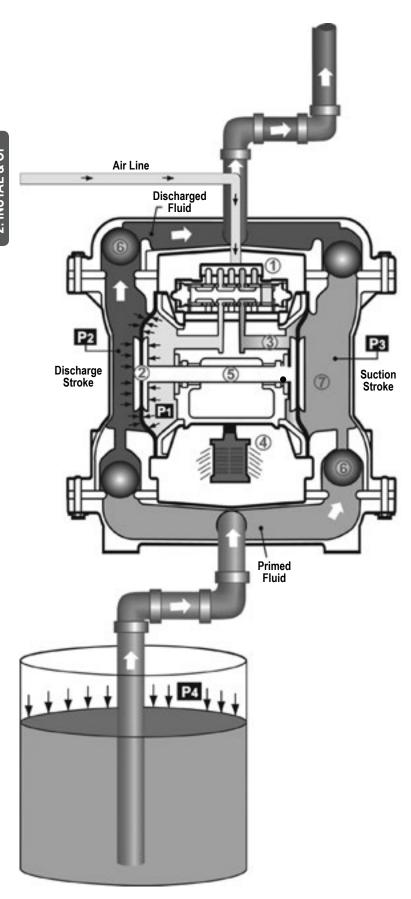
Air-Operated Double Diaphragm (AODD) pumps are powered by compressed air.
