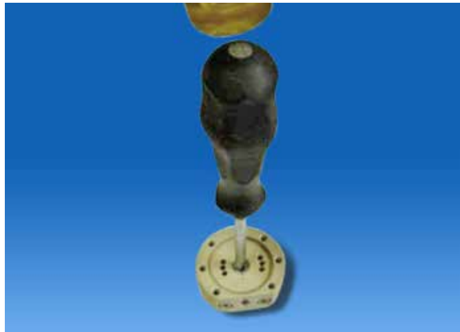
2. Force flat blade screw driver with light blows of the hammer into needle packing.
