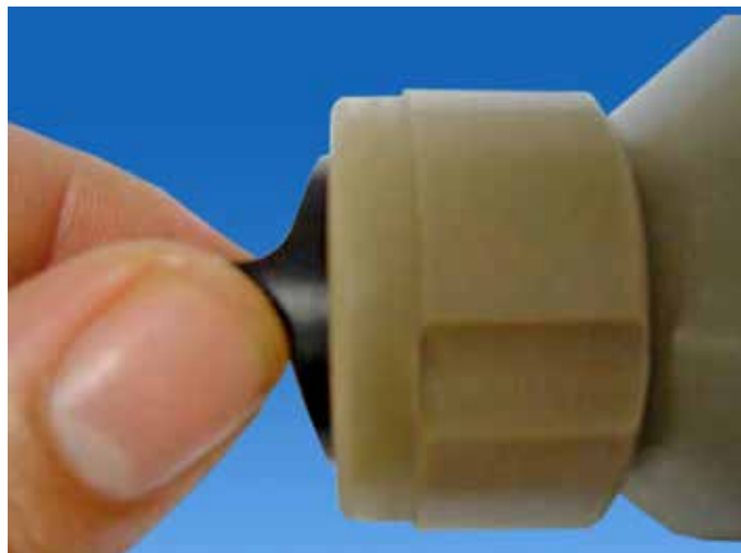
20. Check the position of the air cap while screwing the retaining ring on.
