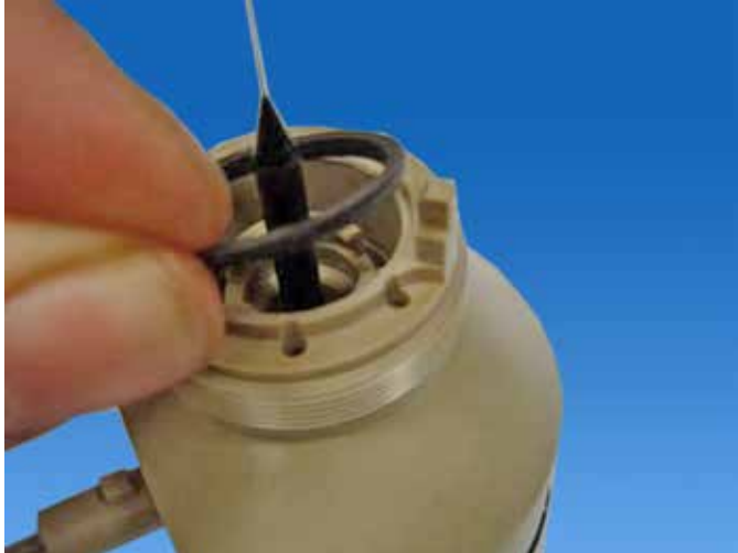
17. Insert disc washer with tapered side into the groove of the baffle.
