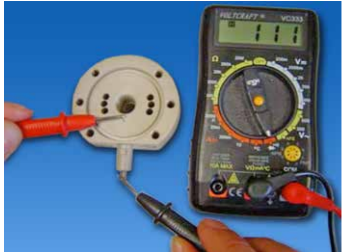
7. Check the electrical contact between wire and cap screw
