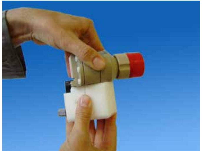
3. Push the gun downward against the spring force until it bottoms on the adapter
