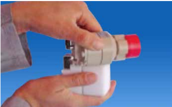
3. Push the gun downward against the spring force until it bottoms on the adapter.
