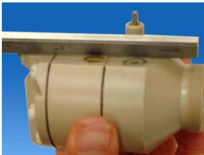
16. Check for levelness with the calliper gauge
