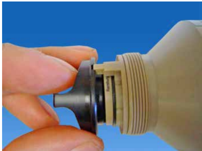
19. Insert the slots of the air cap into the horns of the baffle.
